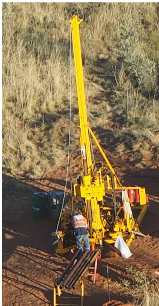
Figure 2 – Heli-supported diamond drilling in progress at Paterson North
