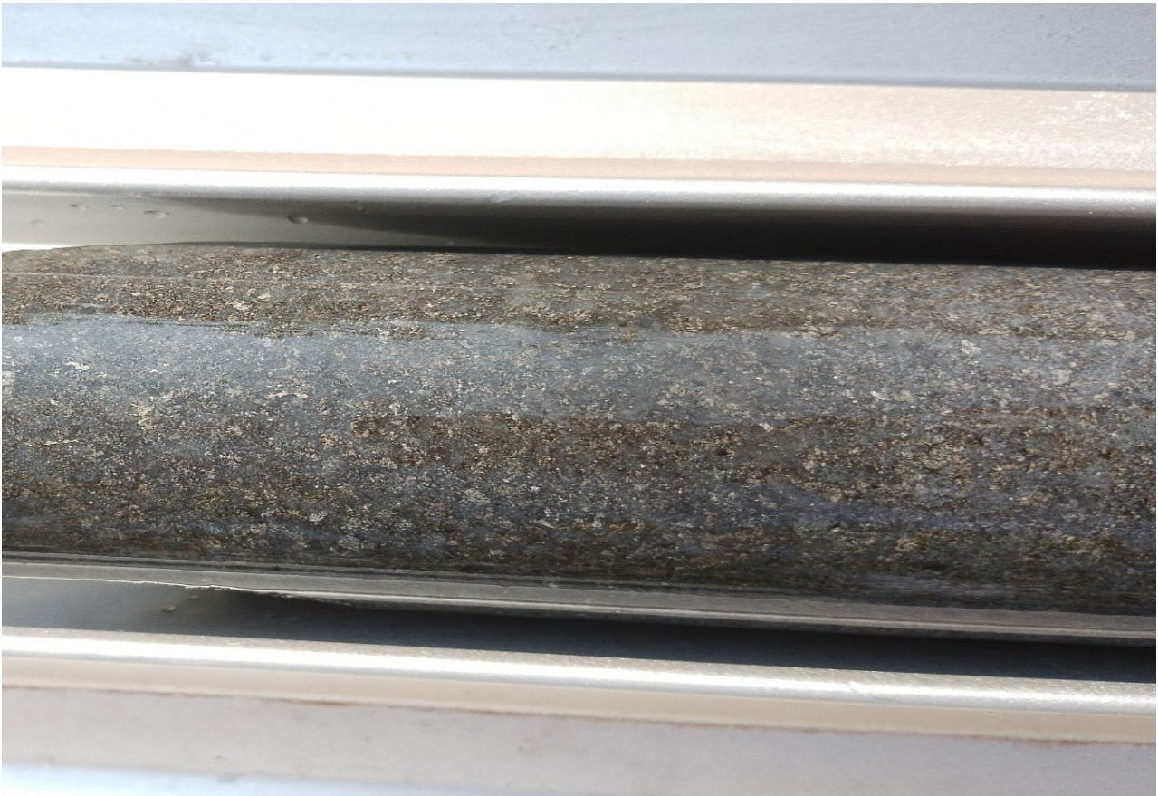
Figure 2: Initial diamond drillhole core showing mafic rock at Liparamba in which disseminated sulphides have been identified at 40m down hole 2 .
