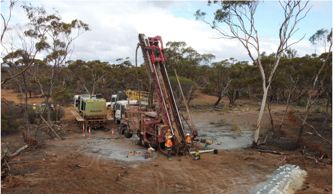
Figure 2. Profile RC drilling rig setup at the Manna Lithium Project.
