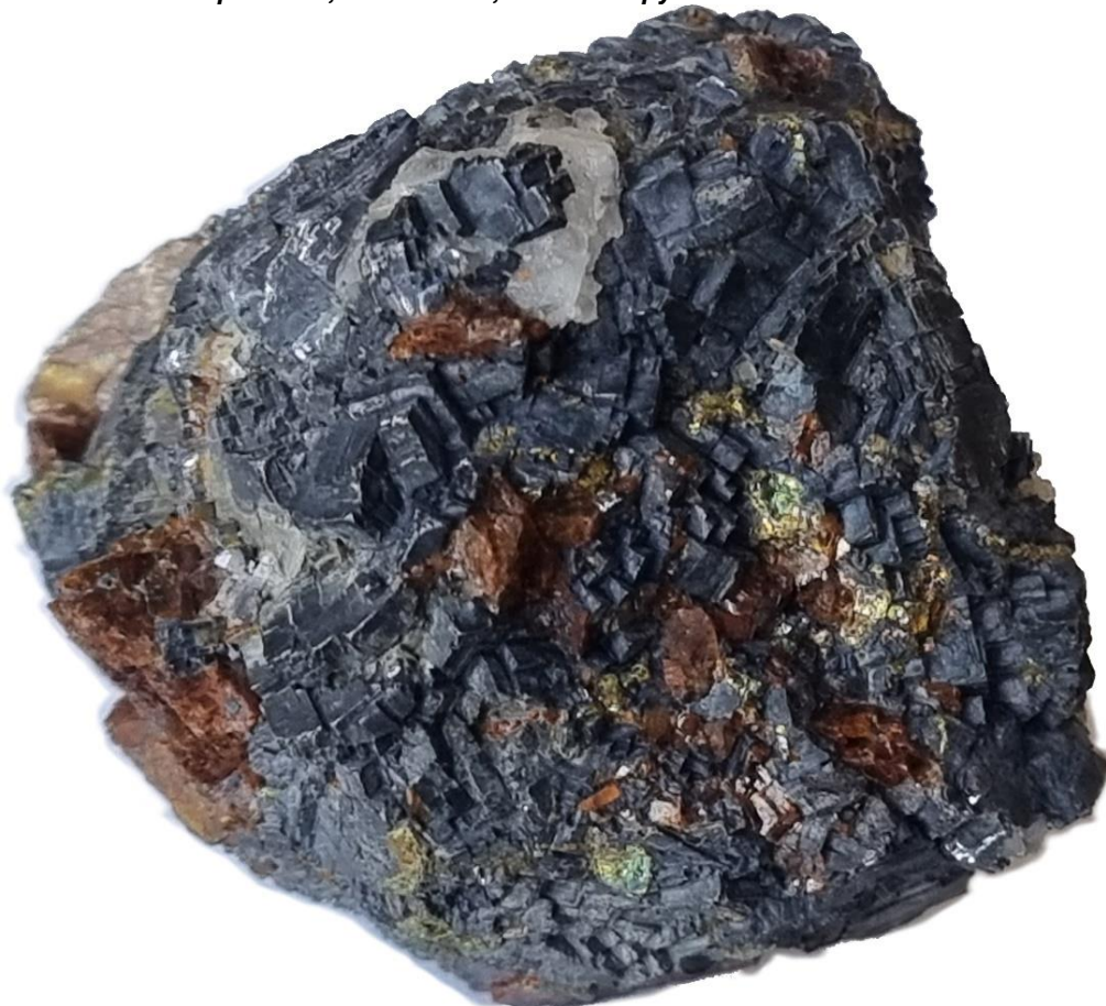
Figure 4. Mineralised waste dump specimen visually estimated to consist of 70% Galena; 10% Chalcopryrite; 10% Sphalerite and 10% Quartz
