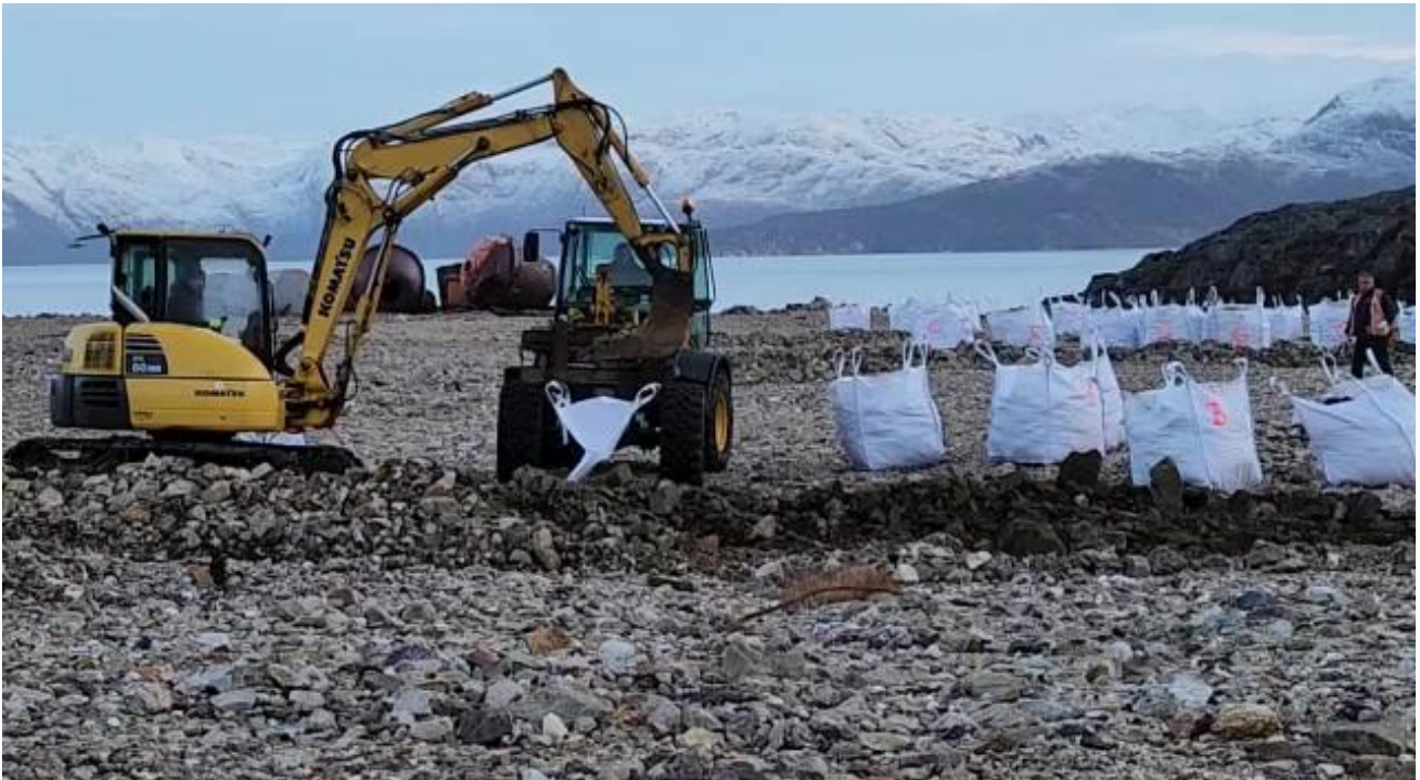
Figure 2: Collecting several tonnes of bulk samples from 5 trenches in the mineralized waste dumps at Ivigtût in 2022
