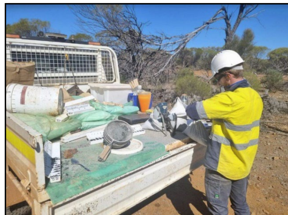
Figure 5: Collecting the cone splitter sample from the RC cyclone
