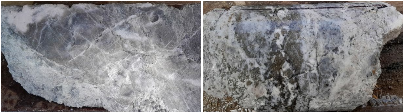
Left: Plate 1. CVDD23-105: 131.8m- Resbolosa brecciated rock with irregular quartz veinlets, and filling of quartz inside the fractures. Right: Plate 2. CVDD23-106: 128.2m- Resbolosa mineralised vein with pyrite and sphalerite sulphide mineralisation.
