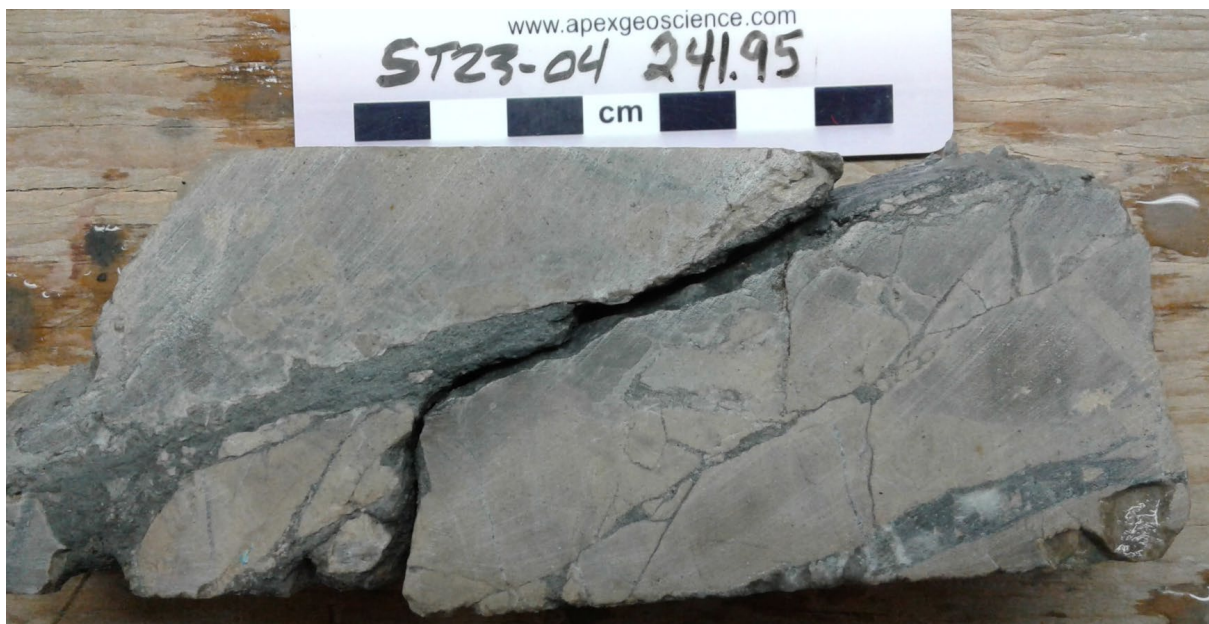
Figure 4: Silt and calcite (darker grey and white respectively) fracture fill within the Southern Graben Fault Zone from drill hole ST23-04 (approximately 241.95m downhole). The fracture matrix is anomalous in copper and likely contains copper oxides after chalcocite (copper sulphide).
