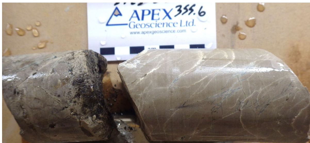
Figure 6: Breccia and veinlets of chalcocite (dark grey) in drill hole ST23-04 from approximately 355.6m downhole.
