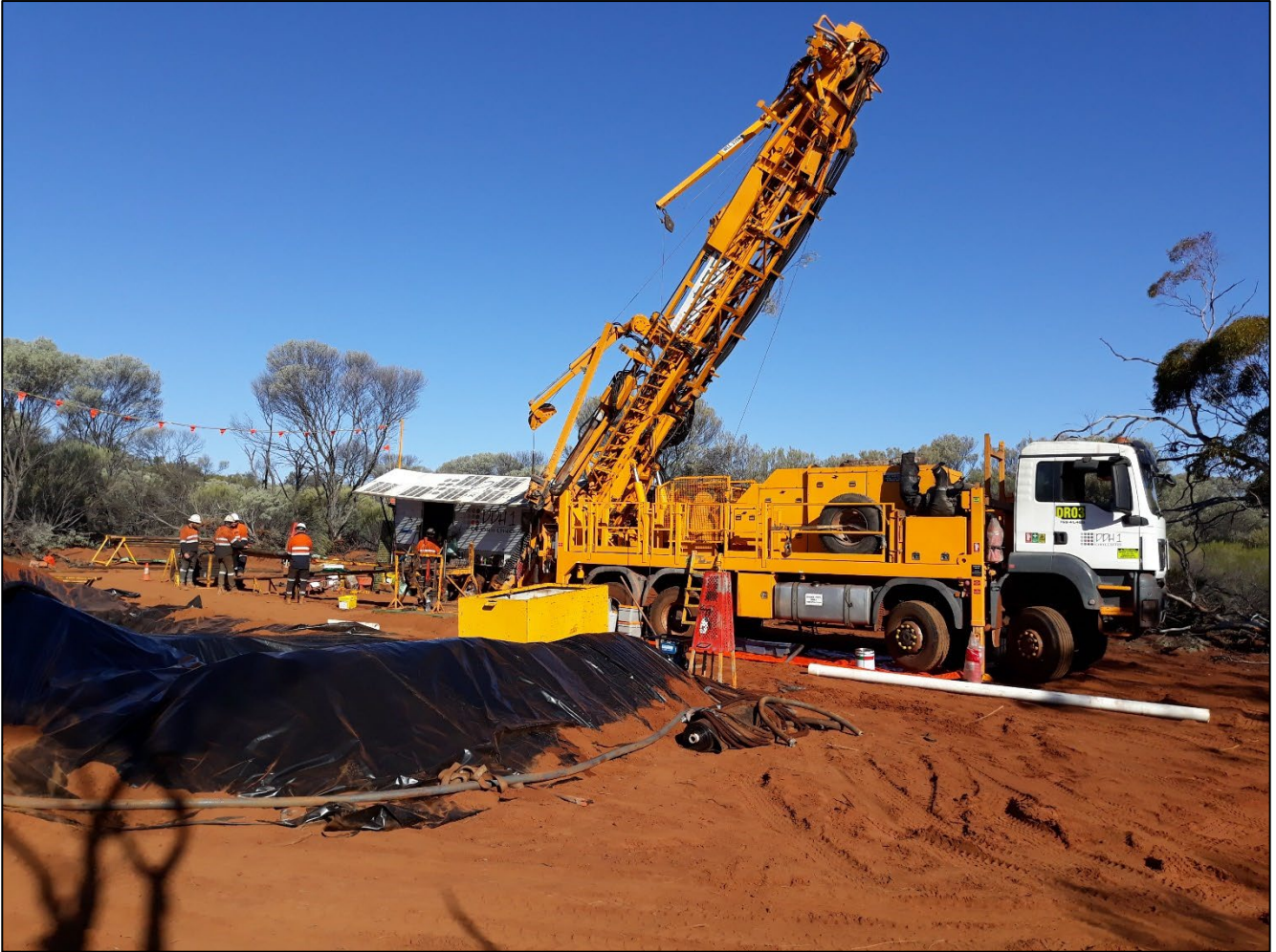
Figure 3: Diamond drill rig supplied by DDH1 drilling AHID0024 at the Highway prospect.
