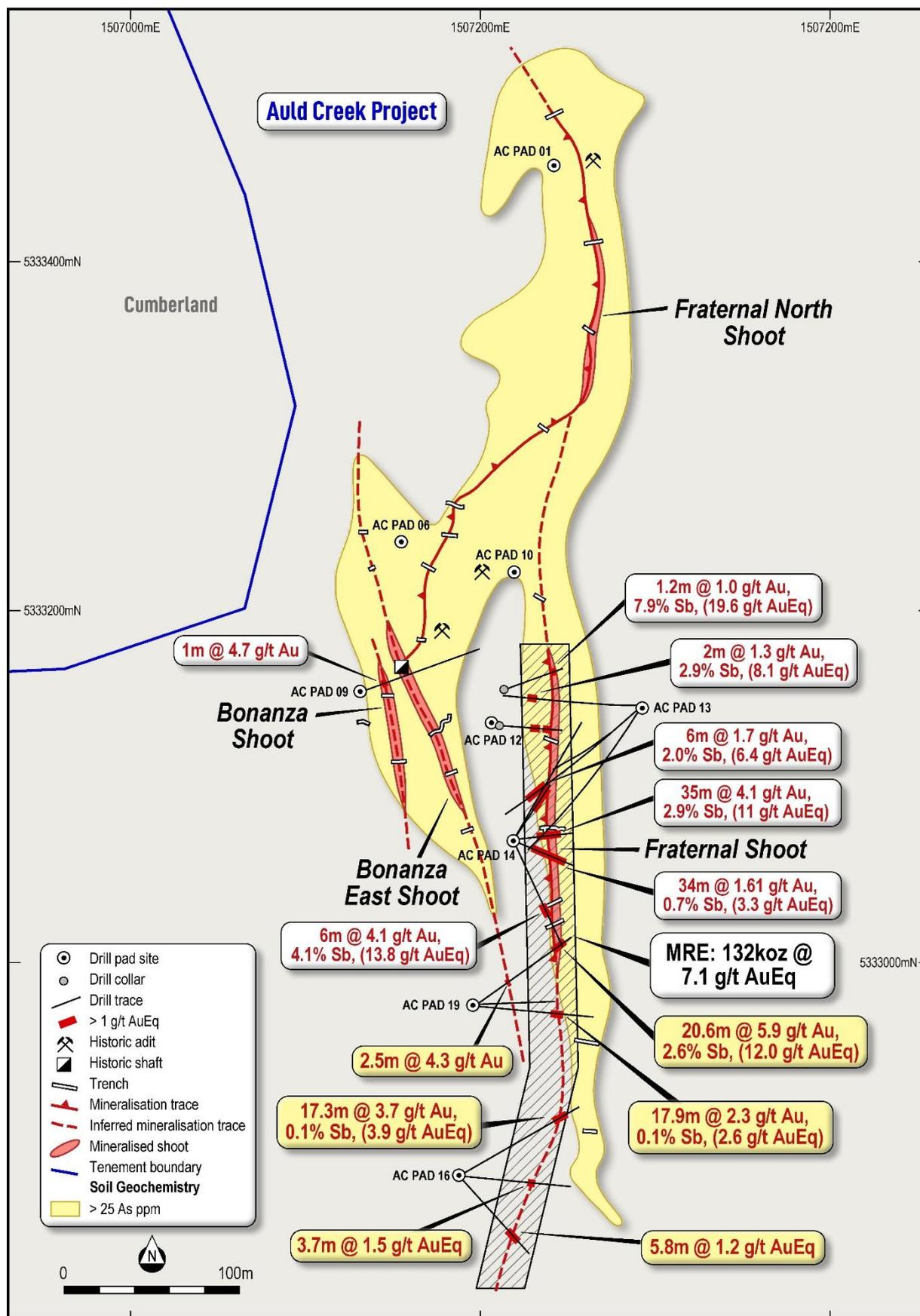
Figure 2. Auld Creek drillhole plan and MRE limits
