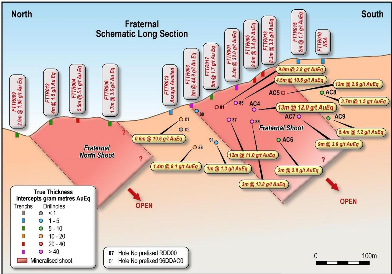
Figure 3. Schematic long section through the Fraternal Zone.
