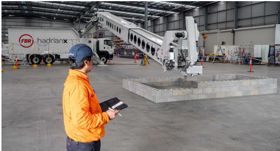
Next-generation Hadrian X® with a new HMI, can be operated by tablet
