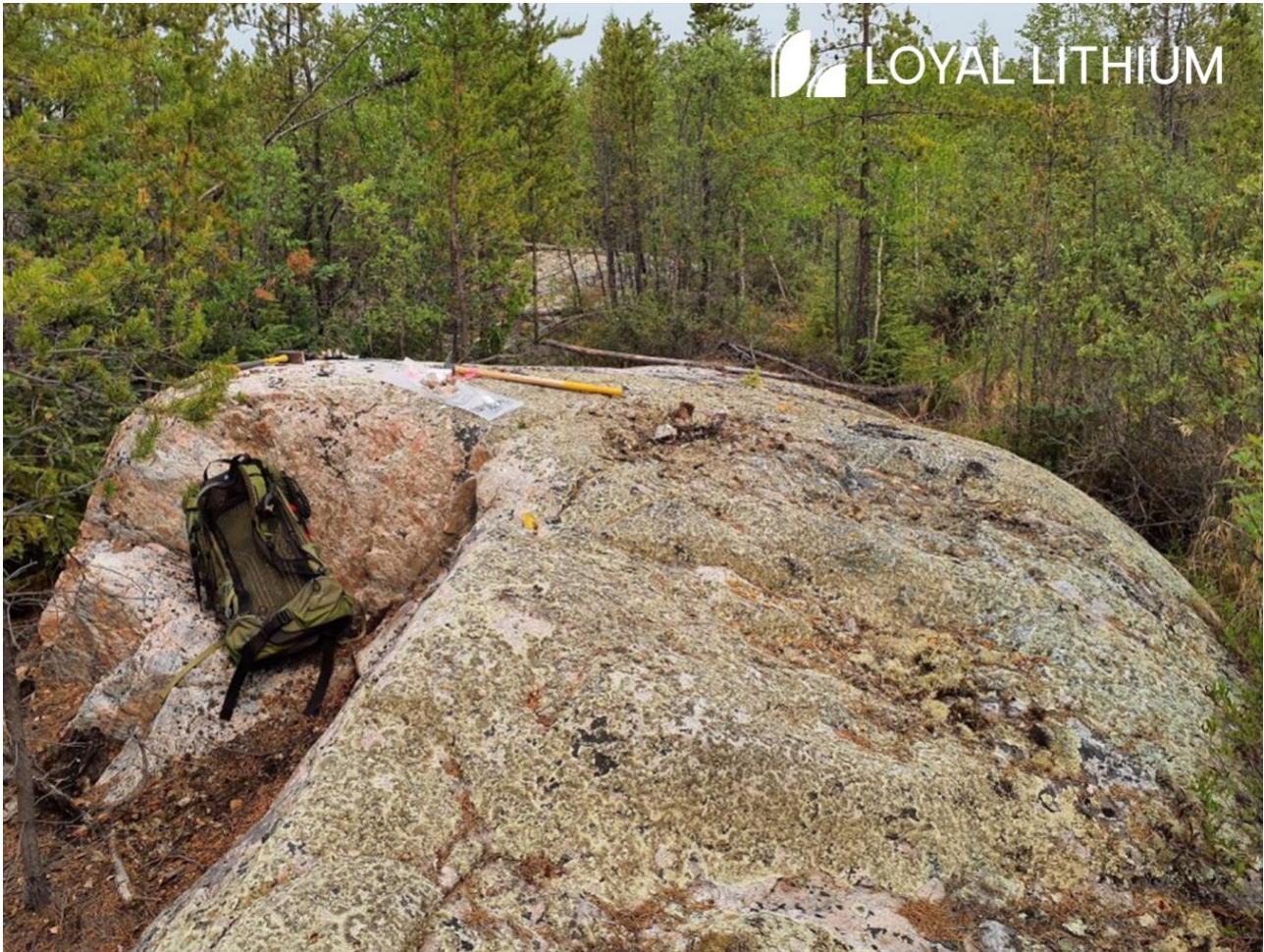
Photo 2: Zone #3, Outcrop Sample D00434032 – D00434034. An in-situ dyke mapped as a spodumene-quartz-feldspar-muscovite pegmatite.
