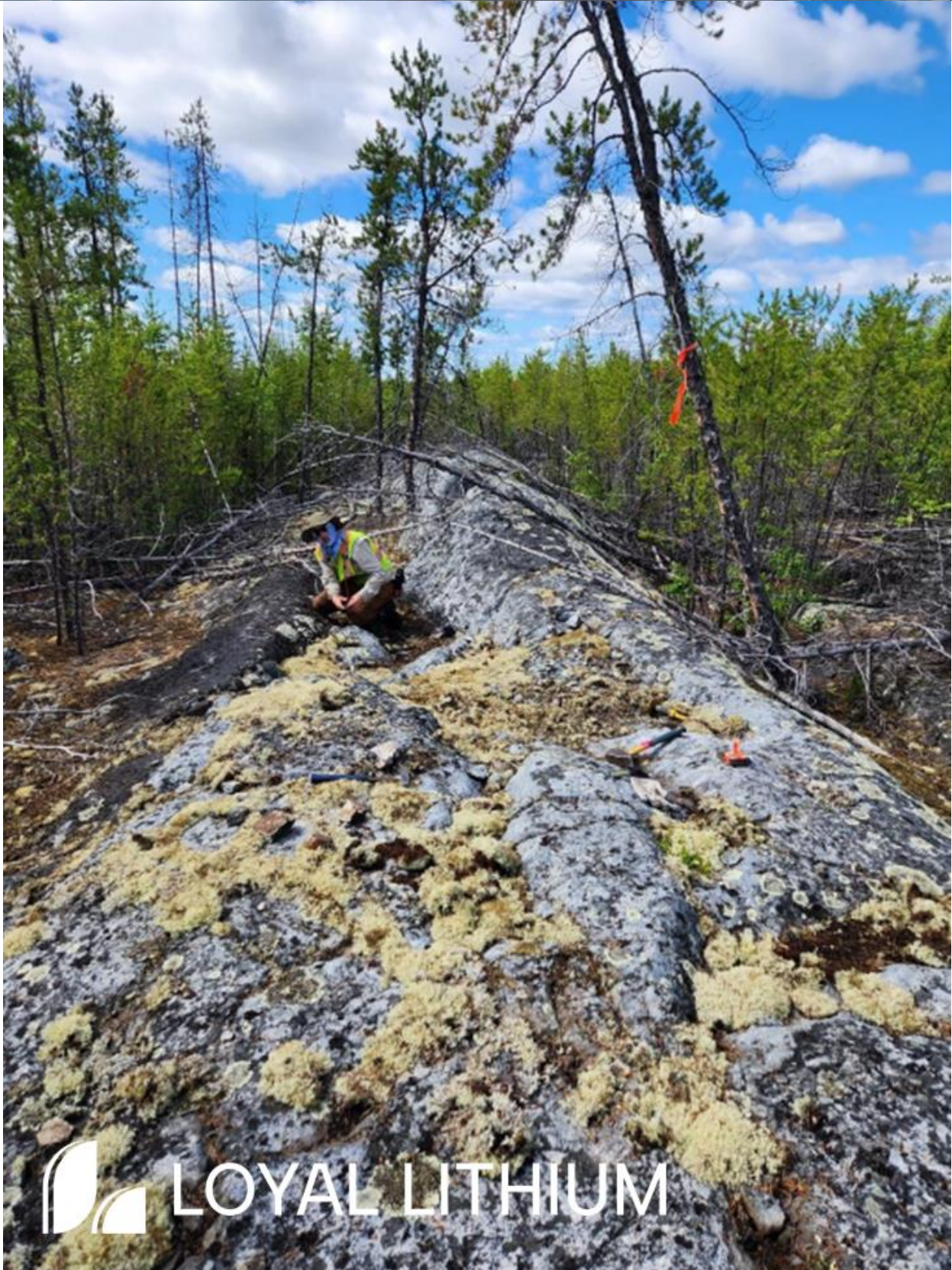
Photo 1: Zone #6 , Outcrop Sample D00434335. An in-situ dyke mapped as a spodumene-quartz-feldspar-muscovite pegmatite. DGC geological field crew inspecting the discovery.
