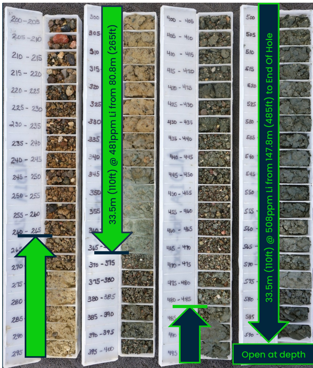
Figure 2. Chip tray samples at 5-foot (Approx. 1.5m) depth intervals from Altair drill-hole AL01 and colour-coded arrows indicating zones of lithium mineralisation.
