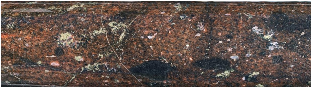
BOD094 – Feldspar-hornblende porphyritic monzodiorite with miarolitic cavities (fossilised bubbles) of calcite-actinolite-chalcopyrite at 1251.7m. Causative porphyry intersection graded 5.5m at 1.62% Cu, 0.82g/t Au from 1249.9m.
