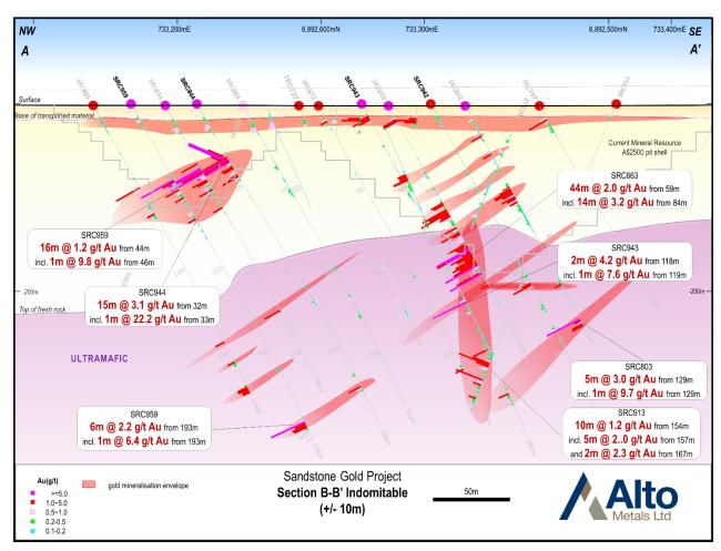
Figure 2: Indomitable section B - B'
