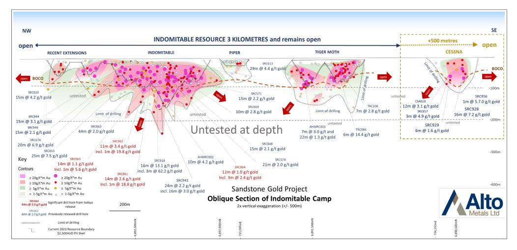
Figure 3: Oblique section of Indomitable Camp showing g/t\*m drill results
