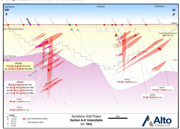
Figure 1: Indomitable section A – A'
