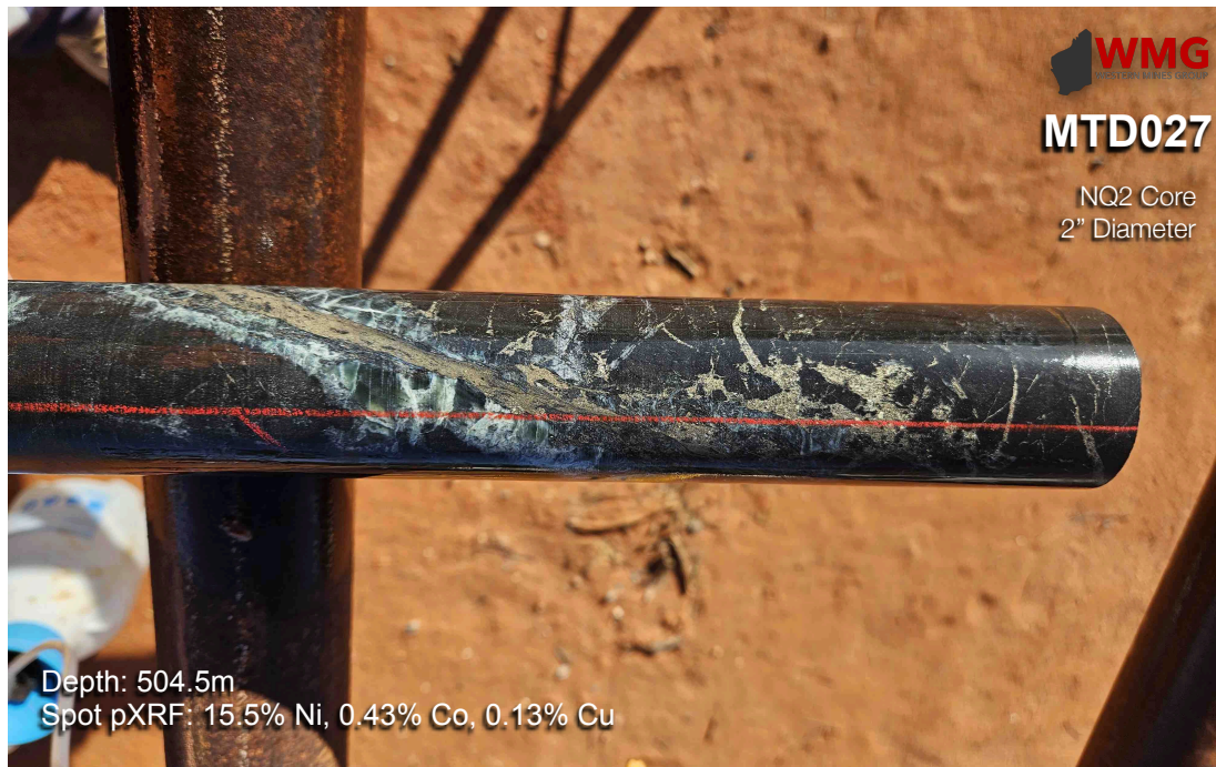
Figure 2: Photo showing high-grade nickel sulphide material filling fractures in hole MTD027 Note: core is NQ2 being 2 inches or 50mm diameter
