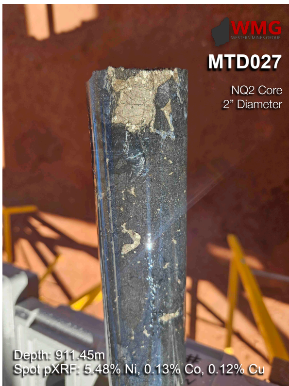
Figure 1: Photos showing examples of remobilised massive sulphide and sulphide globules in hole MTD027 Note: core is NQ2 being 2 inches or 50mm diameter
