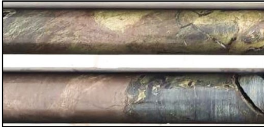
Figure 3 Detail of massive sulphide mineralisation at 190.6m downhole in NRCD293 in top photo with larger interval in lower photo.
