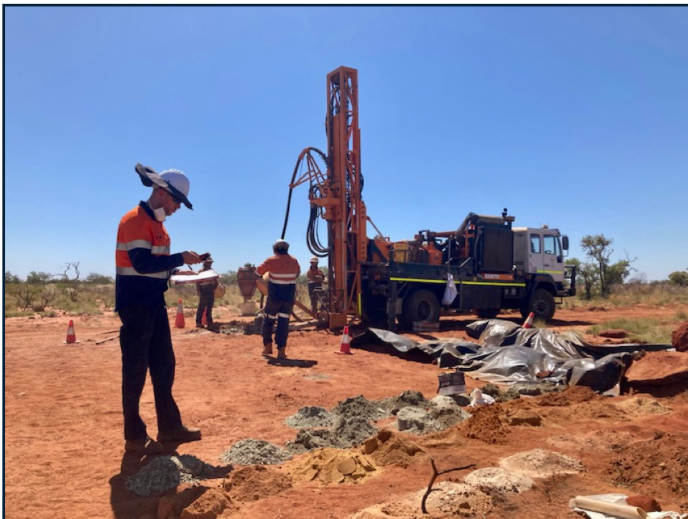
Figure 1: AC drilling at the Yule project's Nomad lithium prospect.
