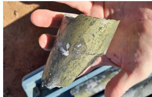
Figure: KSNDH015 - 71.9m: Chalcopyrite vein. Sample interval 71.6m to 72.3m: 5.5% Cu, 0.5g/t Au, 13g/t Ag (see ASX announcement on 24 August 2022).
