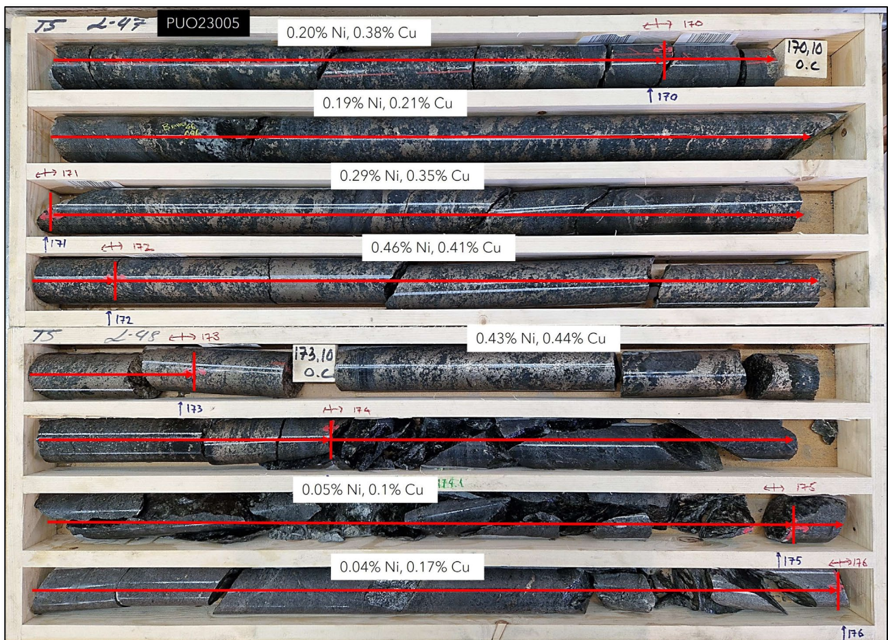
Figure 1: Photograph of drill-core from PUO23005 showing Ni-Cu mineralisation at approx. 169.2-176m downhole.
