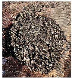
Figure 3: Photo of massive sulphide RC chips from 45-46m comprised of 40-50% pentlandite and chalcopyrite.
