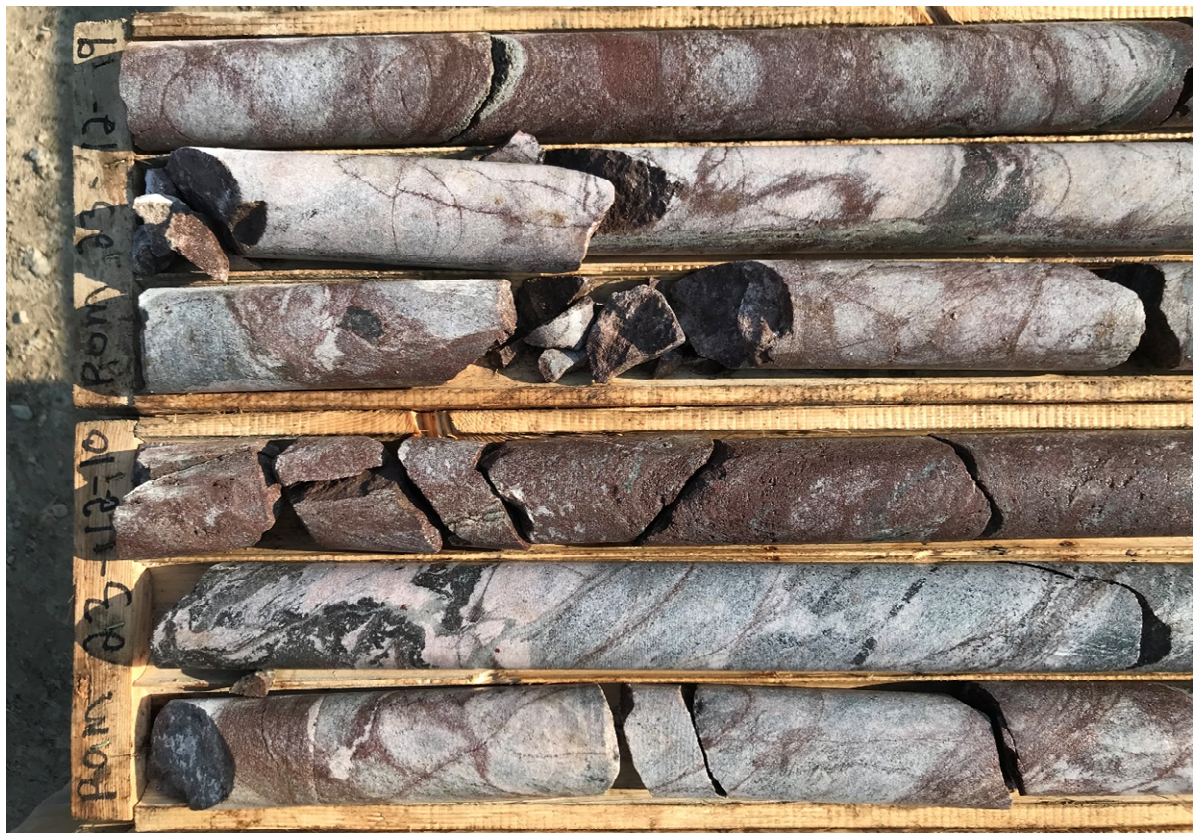
Figure 4: Diamond drill core (NQ, approximately 4.8 cm diameter) from hole POM-23-12 containing abundant visible REE mineralisation (dark red color) hosted in calciocarbonatite. Approximately 56m to 65m down hole.
