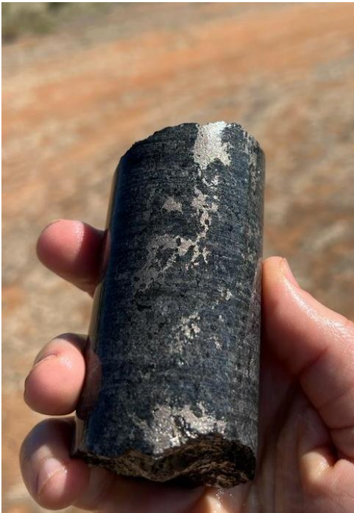
Figure 1. Nickel-Copper sulphides in Diamond drilling from the first hole at Bow River Project at 368m depth.
