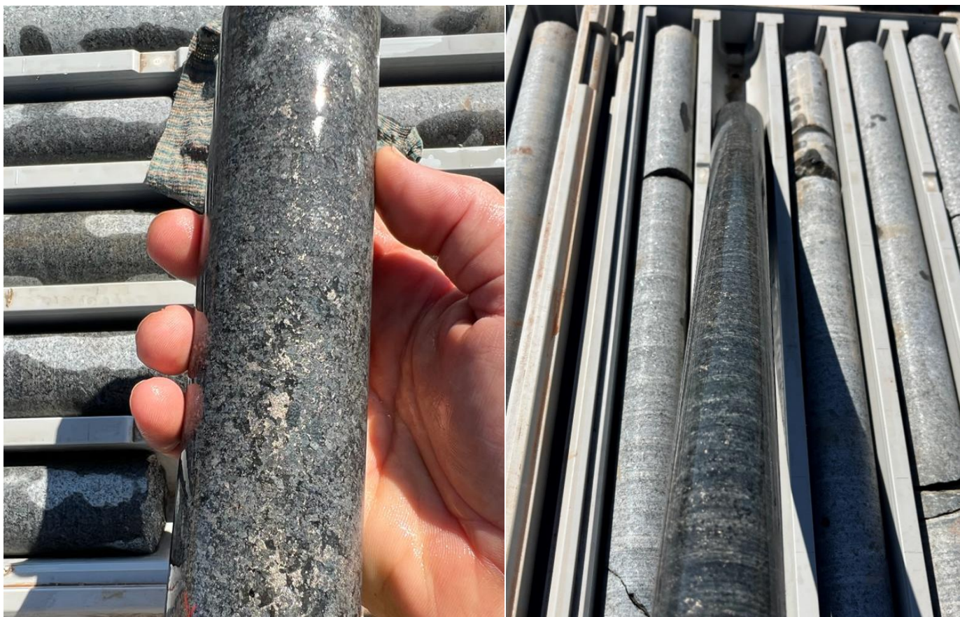
Figure 2. Photos showing examples disseminated and blebby sulphides in hole BRDD001. (Left) Blebby sulphides at 396m, (Right) Disseminated sulphides 397.2m Note core is NQ2 being 2 inches or 50mm in diameter
