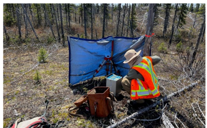
Figure 8 – Geologist on the ground conducting Micro-Gravity survey
