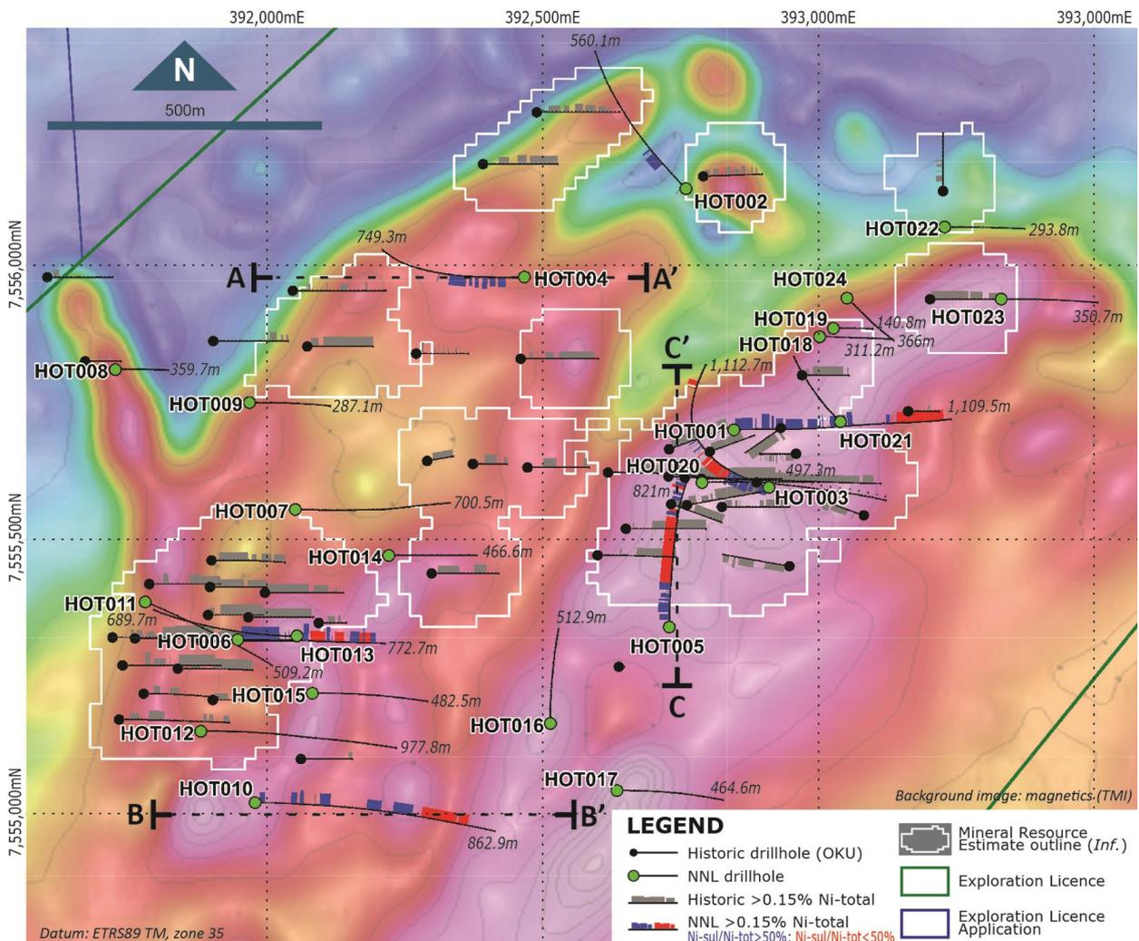
**Figure 2:** Collar plan showing Nordic Nickel’s drilling (green dots) and historical drilling (black dots). Composite assay intersections highlighted (cut-off: >1,500ppm Ni-total; max. 6m internal dilution).
