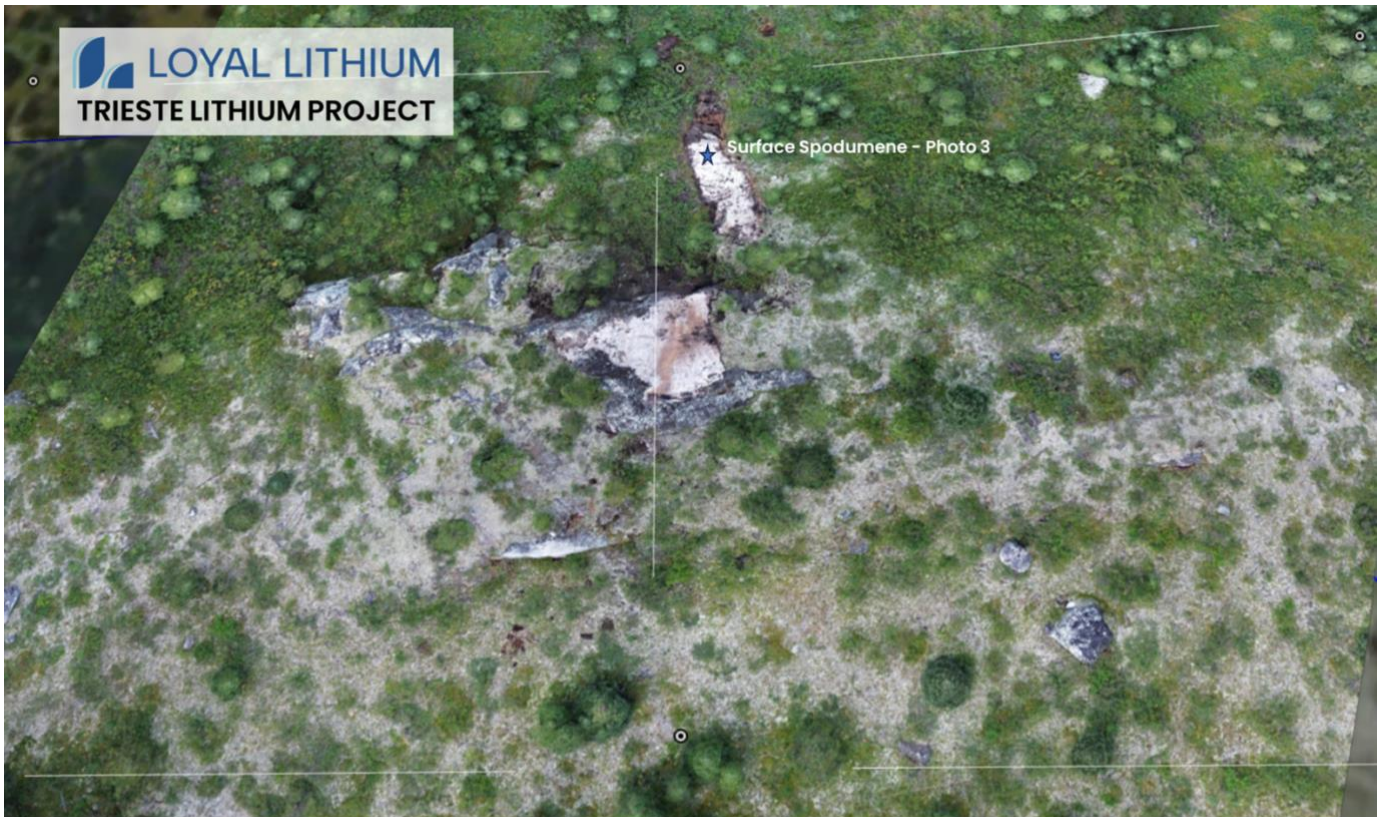
Photo 1: Dyke #01, outcrop TR23AS-15 & 30. A large, prominent weathering-resistant outcrop ridge mapped as a spodumene-quartz-feldspar-muscovite pegmatite. Photo view to the southwest, with an A-Star helicopter shown in the west and geologist traversing the dyke in the centre.
