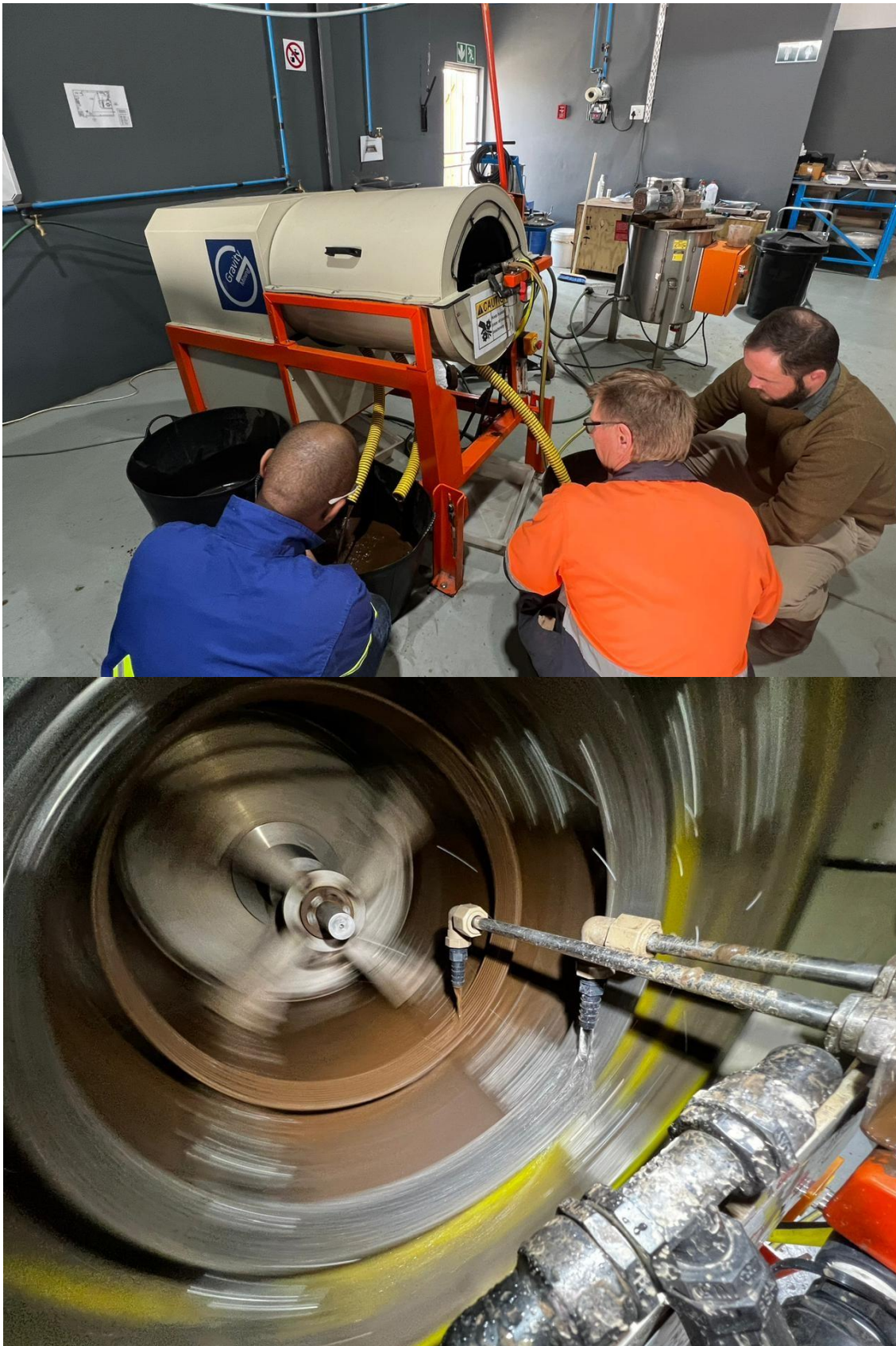
Image 2. Multi-Gravity Separator Testing at Coremet in South Africa. (Top: MGS 900 test machine. Bottom: MGS 900 machine processing Kangankunde mineralisation)
