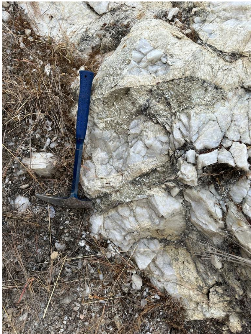
Figure 4: Outcropping pegmatite with altered spodumene (displaying Muscovitization)
