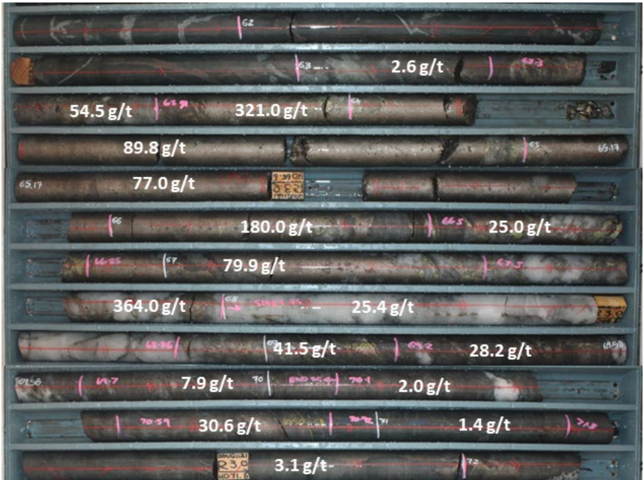
Figure 3: Deacon Main, drillhole DDUG1121 14m @ 49.4 g/t gold, showing zones of high pyrrhotite ore associated with high gold grades, the geology in the infill drilling is analogous to current mining in the Bellevue South area located 400m in the hanging wall of Deacon.
