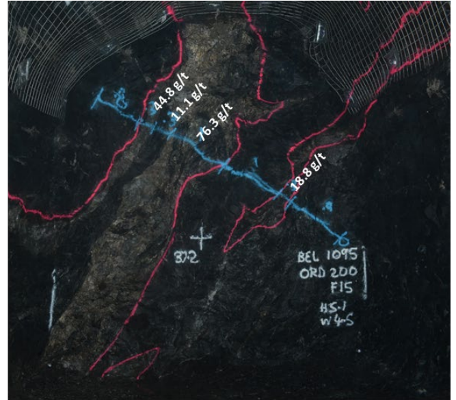
Figure 4: Recent development from the Bellevue South mining area at the 1095 level; consistent zones of high-grade mineralisation associated with high pyrrhotite content. The infill drilling has confirmed the Deacon Main area to be analogous to the Bellevue Lode mineralisation. The Bellevue Lode historically produced ~800k ounces @ 13 g/t gold.
