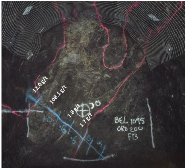
Figure 4: Recent development from the Bellevue South mining area at the 1095 level; consistent zones of high-grade mineralisation associated with high pyrrhotite content. The infill drilling has confirmed the Deacon Main area to be analogous to the Bellevue Lode mineralisation. The Bellevue Lode historically produced ~800k ounces @ 13 g/t gold.
