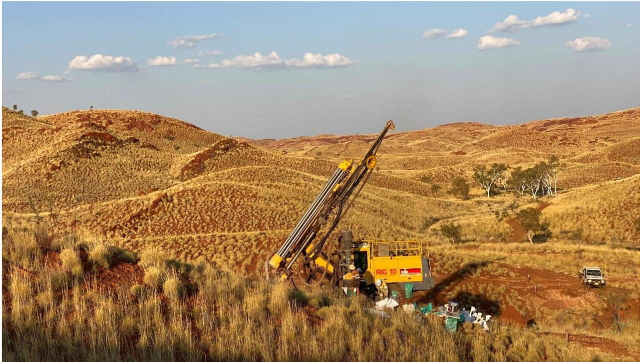
Figure 1: RC drilling underway at Nunyerry North.
