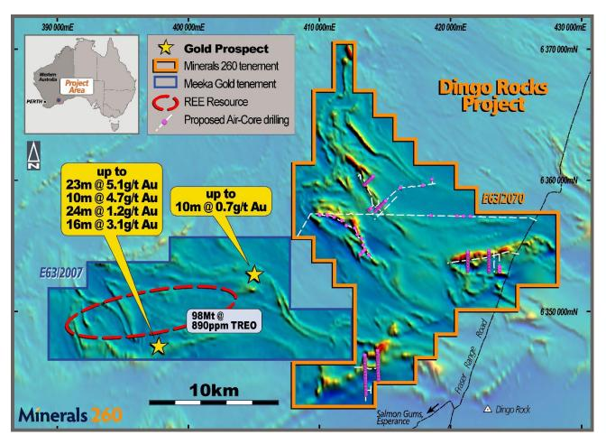
Figure 2 – Dingo Rocks planned Air Core drilling locations with magnetic targets.
