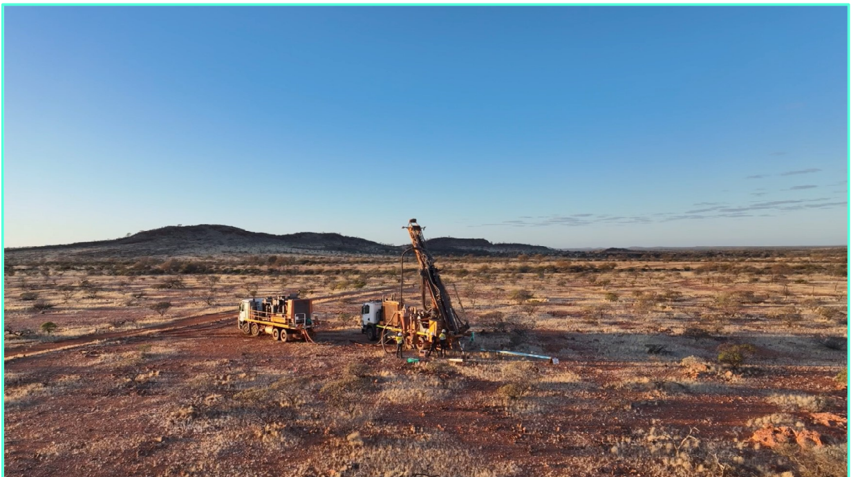
Figure 2. RC drilling at the Morpheus prospect area
