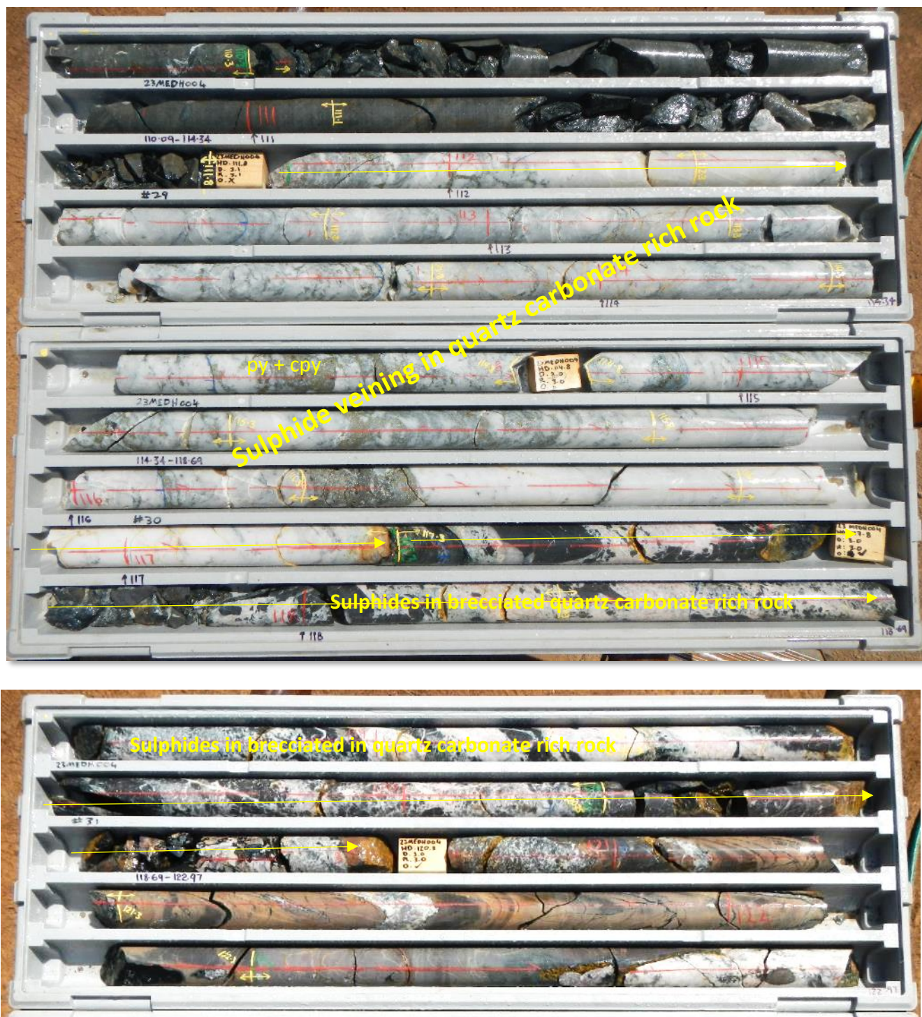
Plate 3: core from drill hole 23MEDH004 (~111m to 121m) showing sulphide mineralisation (see Appendix 2 for more detailed descriptions)
