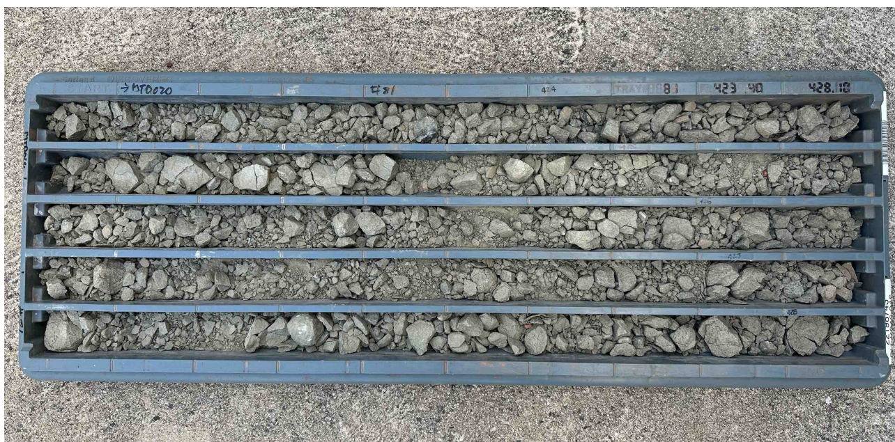
Figure 1C: Mulga Tank Hole MTD020 Tray 81 423m to 428m 11 September 2023 Cut core heavily broken up after 14 months exposure to atmosphere
