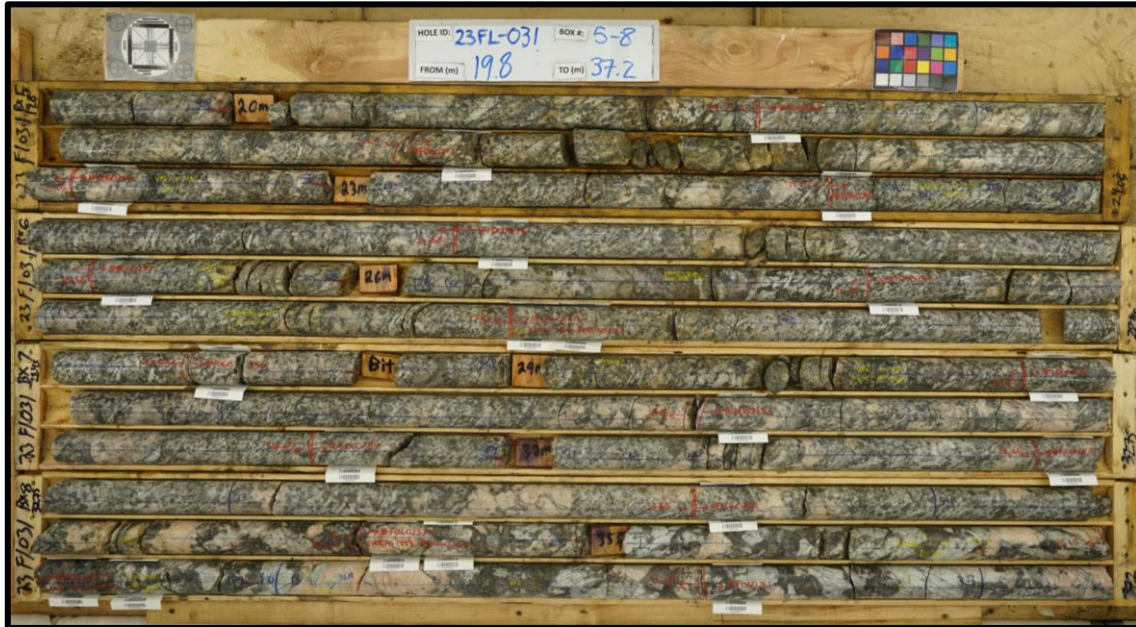
Figure 1 – 23FL-031 Core Box (1.45% Li 2 O over 31.75m)
