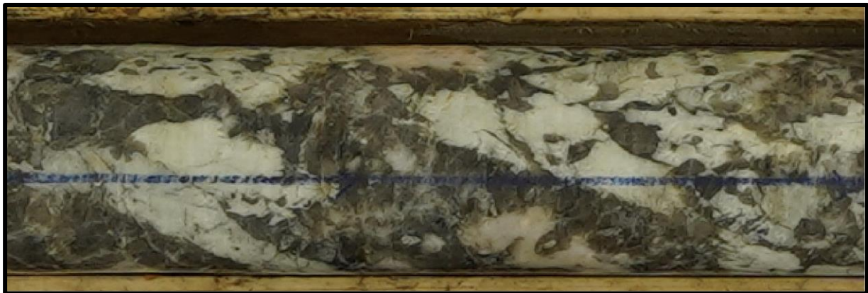
Figure 2 – Spodumene mineralisation in 23FL-018 (2.04% Li 2 O over 8.65m)
