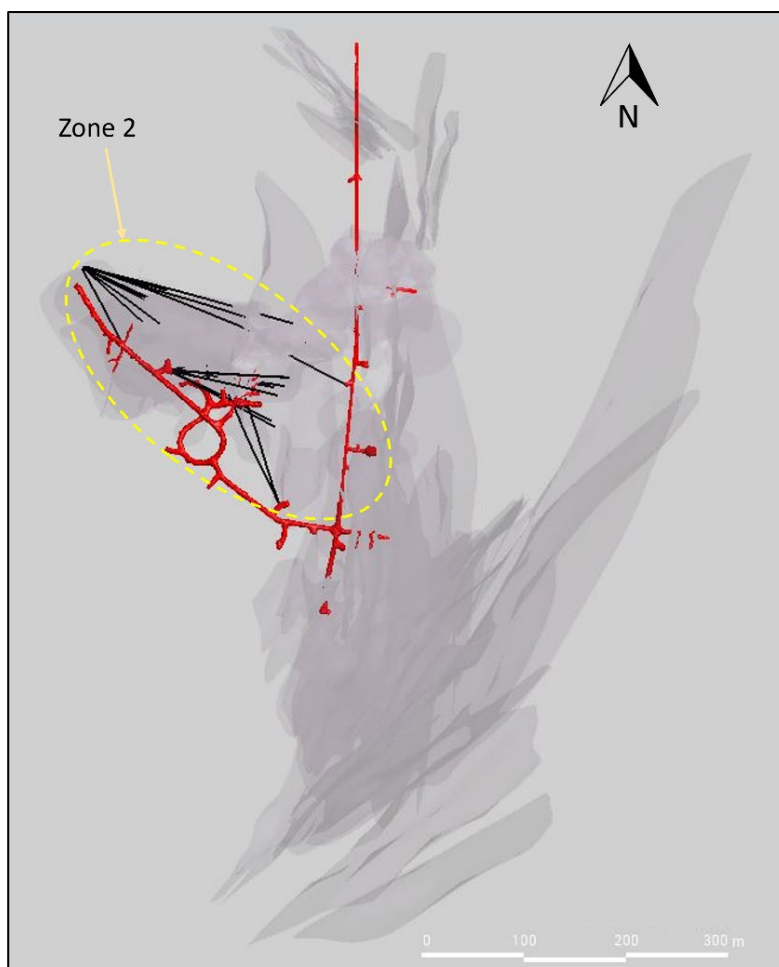
Figure 1. Location of Zone 2 Grade Control Drillholes. Left image: Plan view of Tuvatu showing Zone 2 grade control drillholes in relation to the mineralized lodes. Drillholes are shown in black, mineralized lodes in pale grey, and underground developments in red. The yellow dashed circle represents the Zone 2 area of the deposit.
