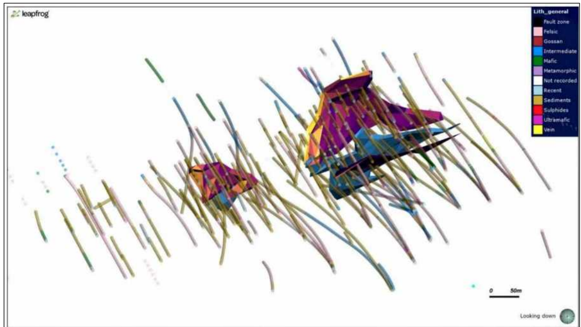
Figure 5.7: Plan view of DD and RC drilling and the interpreted domains for Salt Creek prospect
