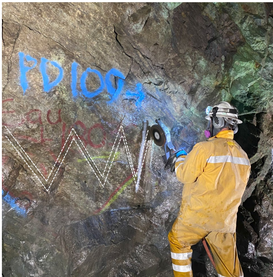
Photo 1 – Example of channel sampling underground walls utilising the “herringbone” sampling pattern. Note sample cut width is approximately 2.5cm
