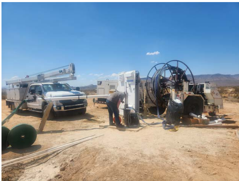
Flow-rate tests in progress on a water well at the Antler Copper Project, Arizona, USA.
