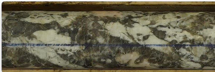
Spodumene mineralisation in 23FL-018 (2.04% Li 2 O over 8.65m)
