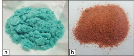
Nickel sulphate (a) and cobalt sulphate (b) produced from Wingellina ores during metallurgical testwork programs
