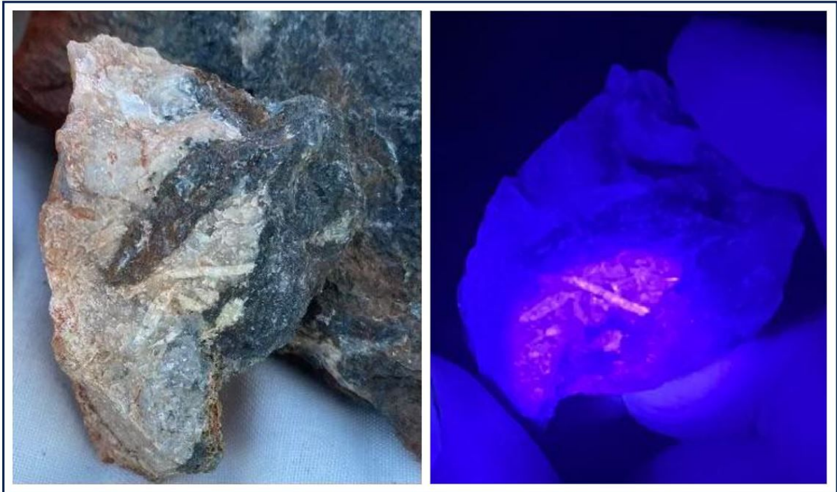
Fig 1 – Hand-specimen of spodumene crystals in LCT pegmatite showing strong pink fluorescence, a characteristic feature under long-wavelength UV light.
