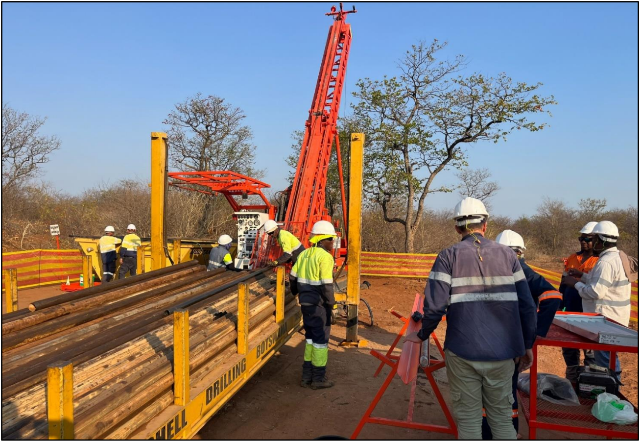
Figure 4: Diamond drilling has commenced at Dibete to test fresh rock AMT anomalies.
