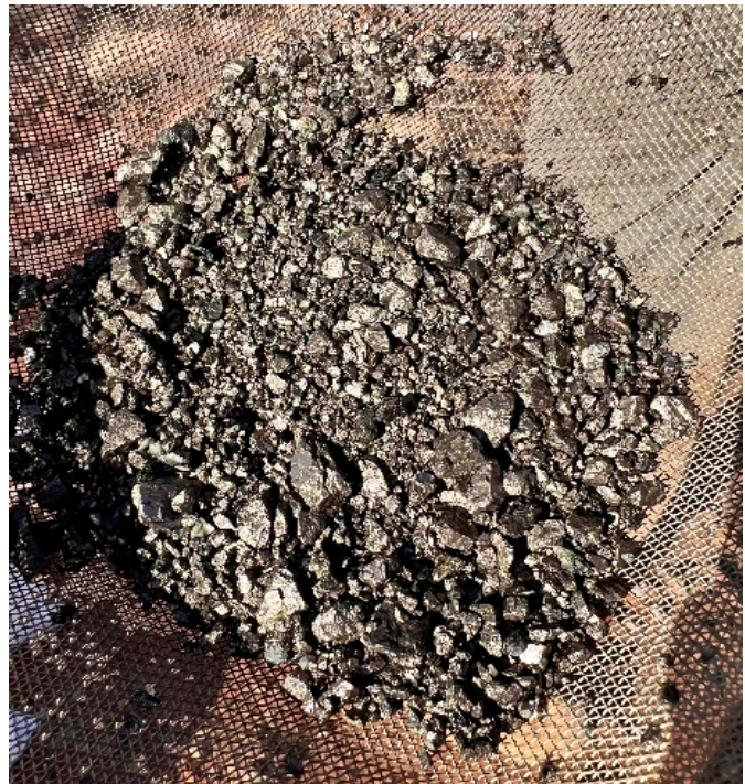
Figure 3: Photo of massive sulphide RC chips from REYRC013 45-46m comprised of 40-50% pentlandite and chalcopyrite.
