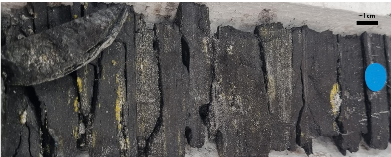
Full-hole core of a Permian coal lithology at the nearby Dunk-1 well
