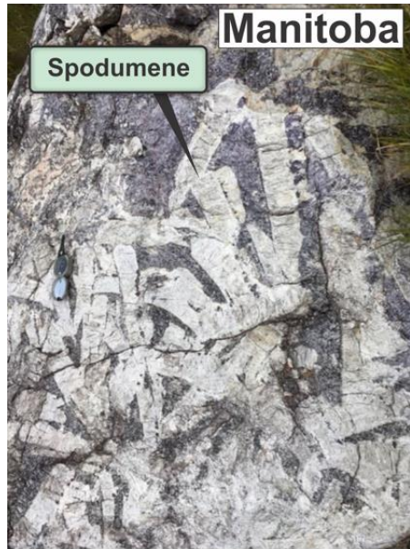
Pegmatite outcrop with abundant white spodumene crystals - Manitoba, Canada https://newagemetals.com/new-age-metals-commences-maiden-drill-program-at-its-lithium-one-project-in-southeastern-manitoba-canada/
