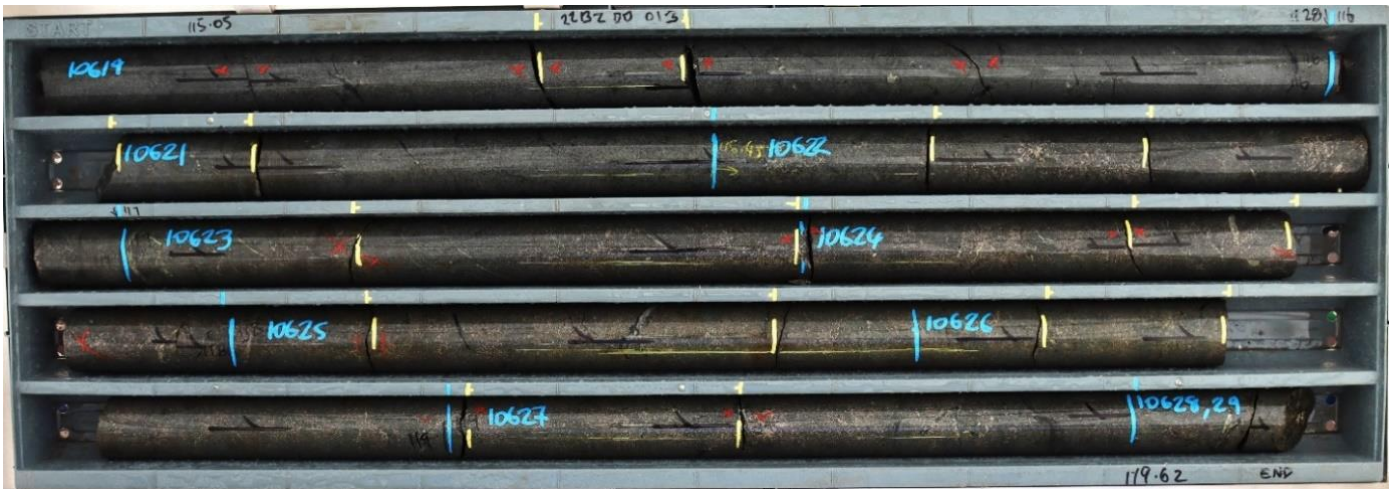
Figure 1: 22B2DD013 (115.05-119.62m – NQ core 47.6mm diameter) incl. 3.1m @ 3.83% Ni Eq from 116.4m Strongly mineralised dolerite with densely disseminated fine-grained pyrrhotite, chalcopyrite, and pentlandite. 5
