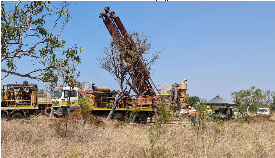
Figure 1: Photo of the RC Rig set up to commence drilling at Tarraji.
