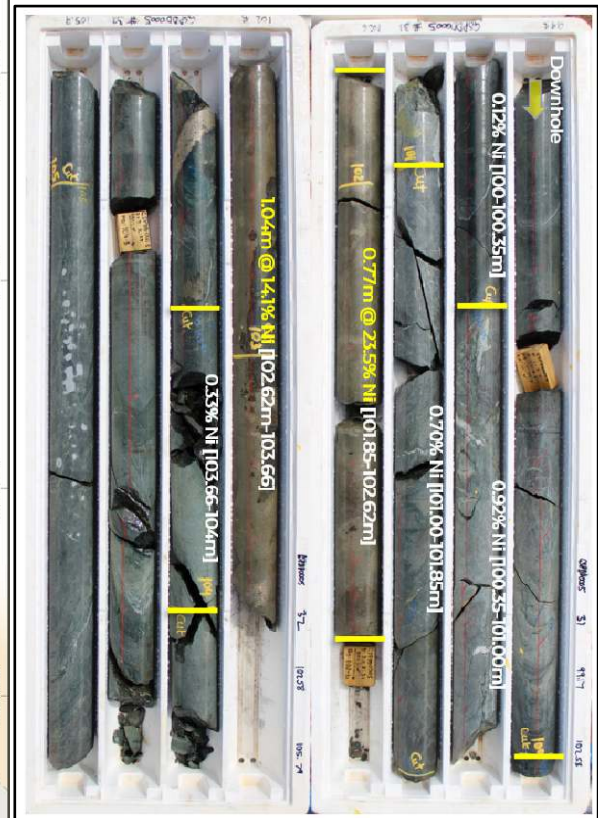
Figure 10: Core photo showing sample intervals through massive sulphides in GSPDD0005. The combined intercept is 18.1% Ni, 19.06g/t Pd, 2.22g/t Pt and 2.21g/t Au.
