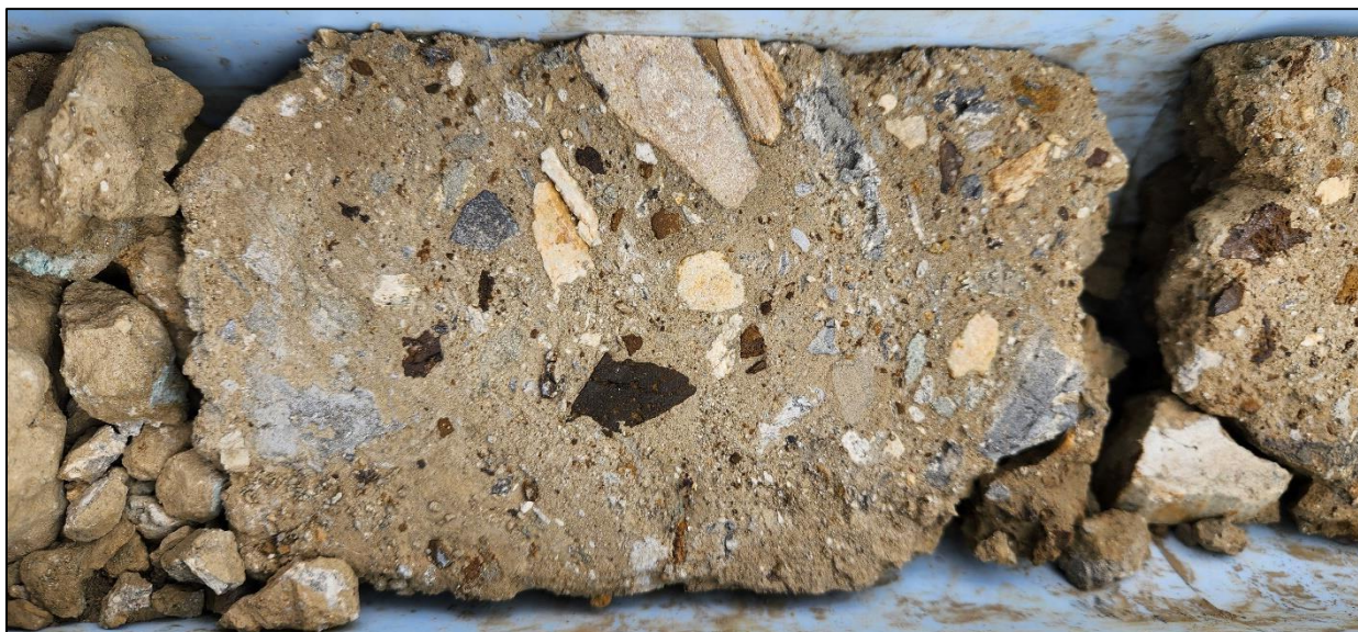
MLJDD020_178.0m_Polymictic Breccia with silica-pyrite clast
