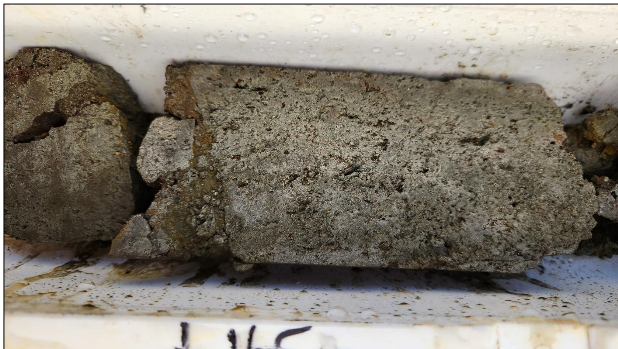
MLJDD018_164.5m_Massive pyrite in Breccia
