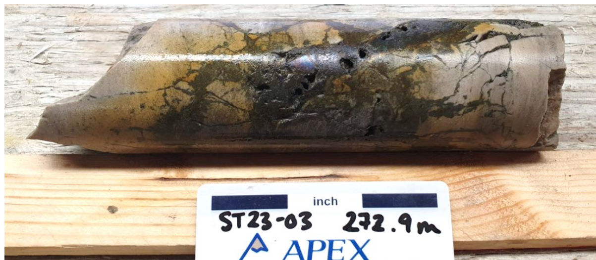
Figure 8: Breccia chalcocite (dark grey), bornite (purple/grey) and chalcopyrite (brassy) in drill hole ST23-03 from approximately 272.9m downhole.
